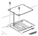
Figure 4-9. Replacing the Memory Compartment Cover
